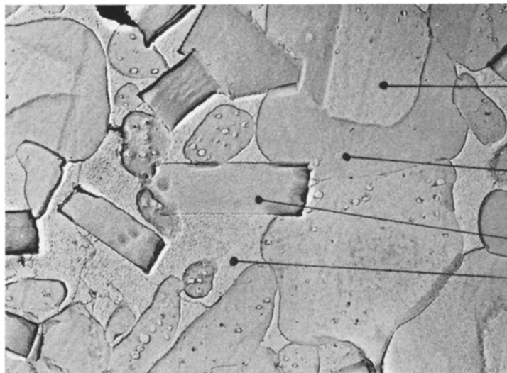
Figure 5 Structure of a sintered (W, Ti) C-Co alloy, electron-micrograph (Mowital replica).
